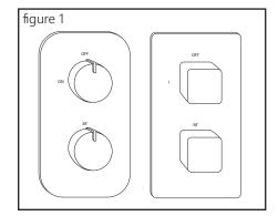
2. Use a thermometer to test the water temperature from one of the outlets. Adjust the temperature by turning the temperature control handle clockwise or anti-clockwise until 38°C is achieved. Remove the handle and re-attach it so it is aligned as shown in figure 1.
