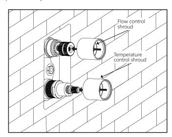
10. Push the backplate onto the flow control 11. Seal the plate to the tiles using silicone and temperature control shrouds.
