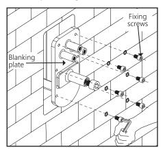
6. Check to ensure that the o-rings are firmly 7. Place the valve body into the ARMERA dock secured in the back of the valve body. If the o-rings are damaged or not seated correctly, the valve body will not seal with the ARMERA dock and leaks may occur.
