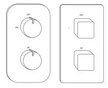
The valve has been calibrated so that 38°C is achieved with the handles positioned as in above diagrams. If water temperature is higher or lower than 38°C, please follow the instructions for recalibrating the thermostat.
