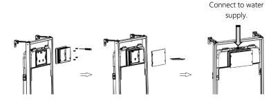
7. Attach the threaded bars from the WC mounting kit. Check to ensure that the width at which the bars are set match the fixing points in the WC that is to be installed. Cover the bars with the protective plastic sleeve to prevent damage occurring.
