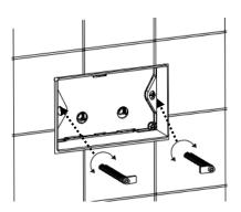
2. Attach the flush plate housing to the flush plate fixings.
