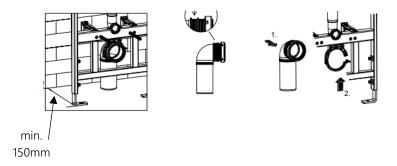
If outlet pipe is offset, please allow min 170mm installation depth.
