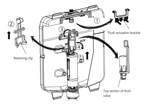
5. The main body of the flush valve can then be removed from the cistern.
