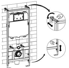
When you are satisfied that the frame is in the correct position and is level, mark the fixing points on the wall and the floor.
