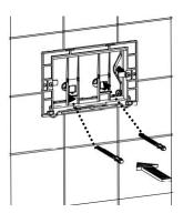
4. Fix the flush plate into position.
