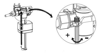
2. If the cistern becomes slow to fill or does not stop filling, the fill valve can be removed and cleaned.
