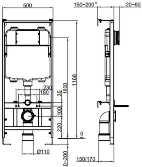
\*NB If outlet pipe runs directly into the wall a minimum depth of 110 can be achieved by attaching the angled bracket directly to the frame:
