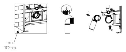
3. Offer the frame up to the wall or studwork onto which it will be attached. Use a spirit level to ensure it is level. Adjustments can be made on each of the 4 wall brackets. The height of the frame can be altered by sliding the feet in or out of the frame.
