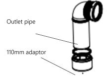
If outlet pipe runs straight down, please allow min. 150mm installation depth.
